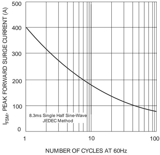
Fig. 3 Maximum Non-Repetitive Peak Forward Surge Current
