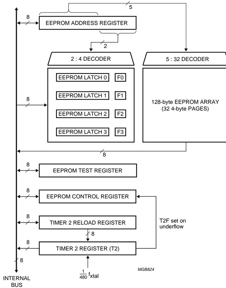
Fig.5 Block diagram of the EEPROM and Timer 2.
