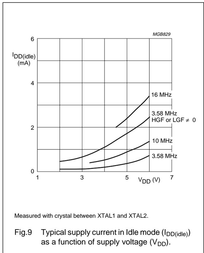
8-bit microcontrollers with DTMF generator and 128 bytes EEPROM
