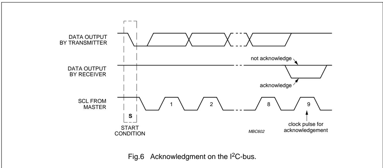
Fig.6 Acknowledgment on the I2C-bus.
