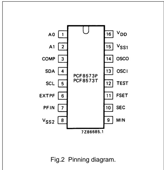
Fig.2 Pinning diagram.
