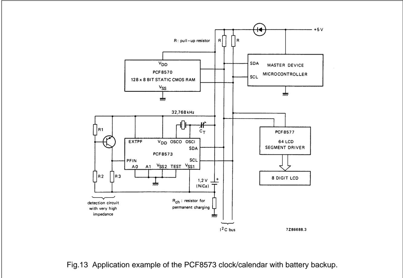
Fig.13 Application example of the PCF8573 clock/calendar with battery backup.
