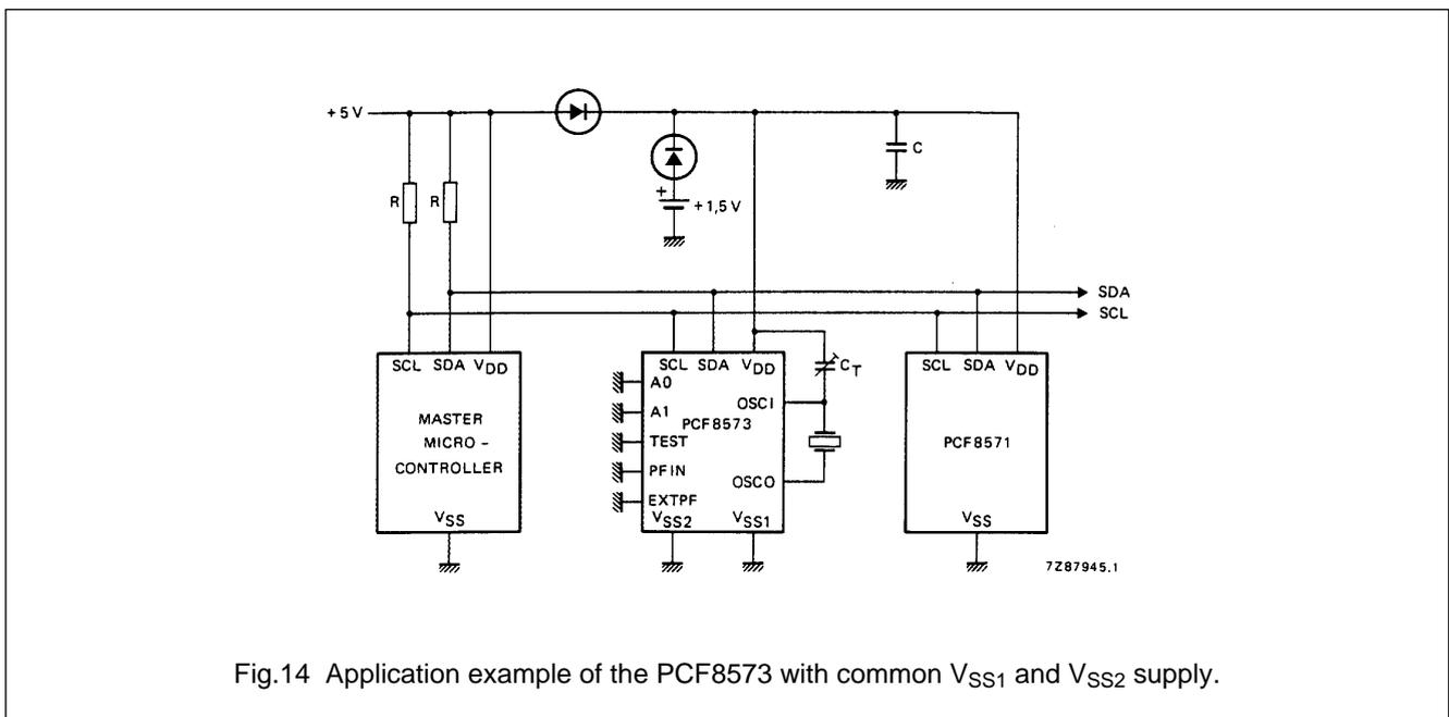
Fig.14 Application example of the PCF8573 with common VSS1 and VSS2 supply.
