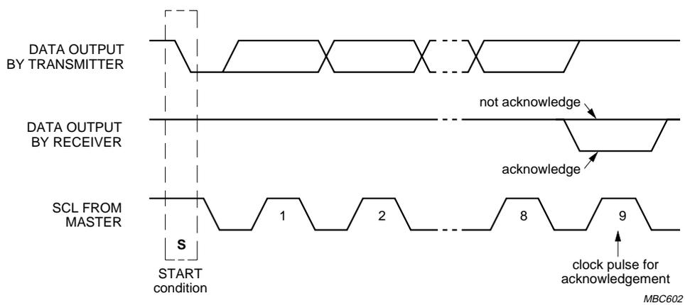
Fig.15 Acknowledgement on the I<sup>2</sup>C-bus.
