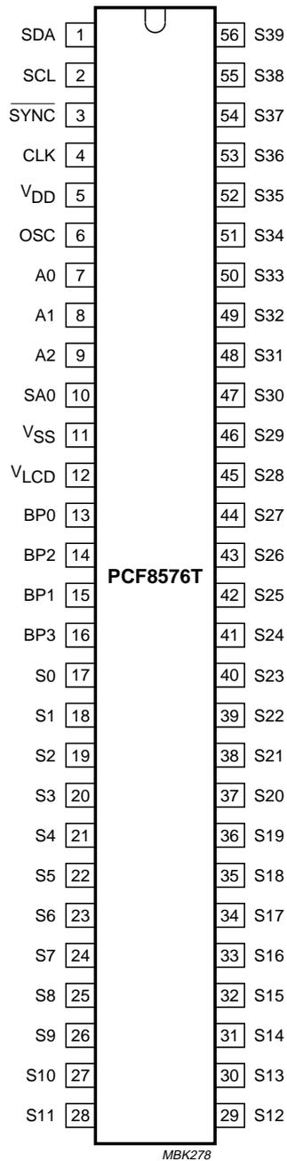
Fig.2 Pin configuration; SOT190-1.
