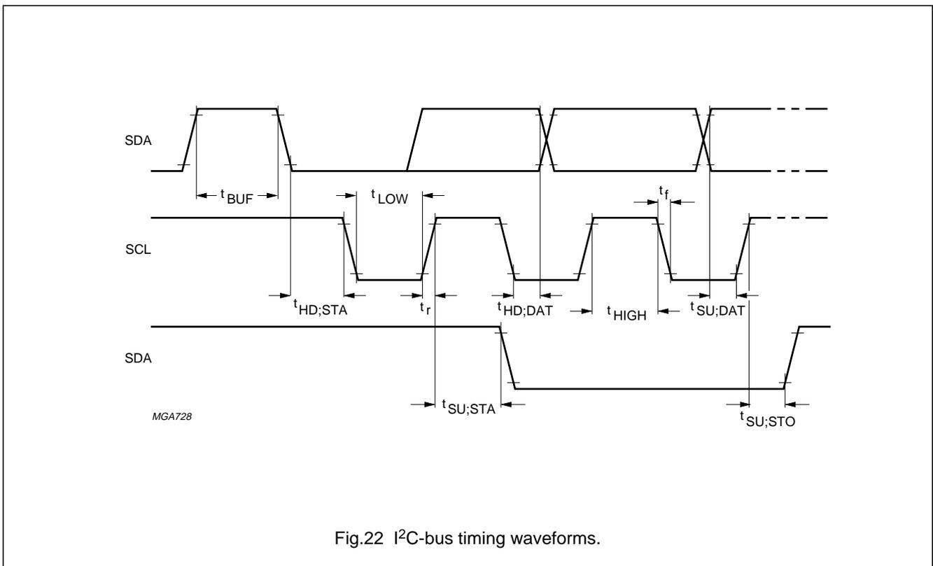
Fig.22 I<sup>2</sup>C-bus timing waveforms.
