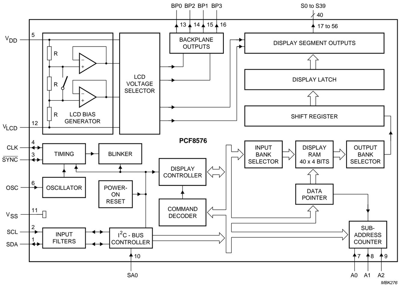
Fig.1 Block diagram (for VSO56 package; SOT190-1).
