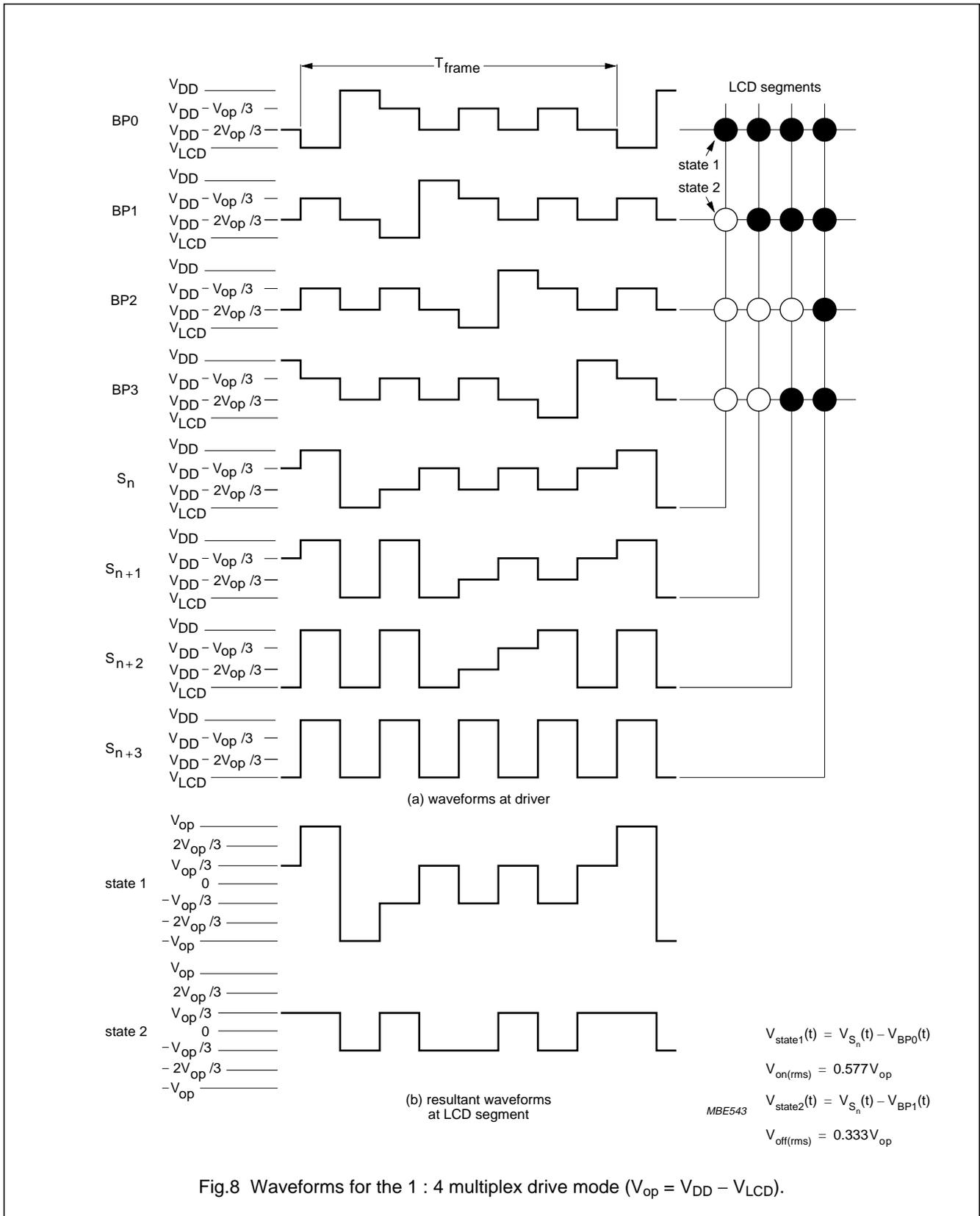
Fig.8 Waveforms for the 1 : 4 multiplex drive mode ( $V_{op} = V_{DD} - V_{LCD}$ ).
