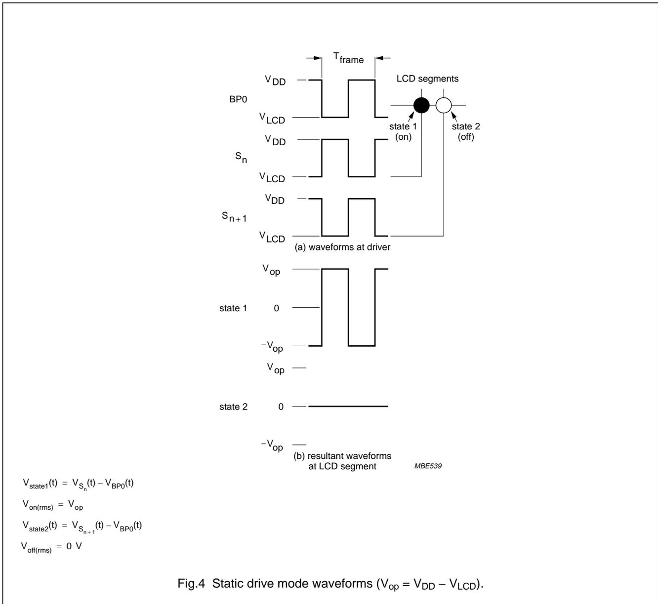
Fig.4 Static drive mode waveforms ( $V_{op} = V_{DD} - V_{LCD}$ ).
