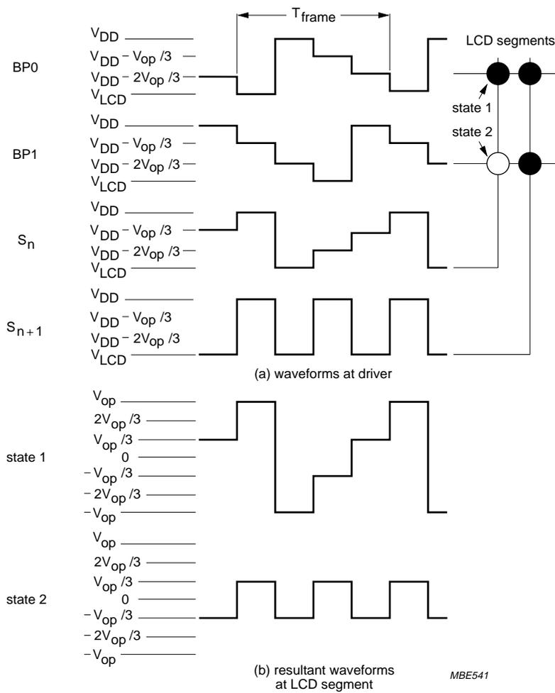
$$V_{state1}(t) = V_{S_n}(t) - V_{BP0}(t)$$
