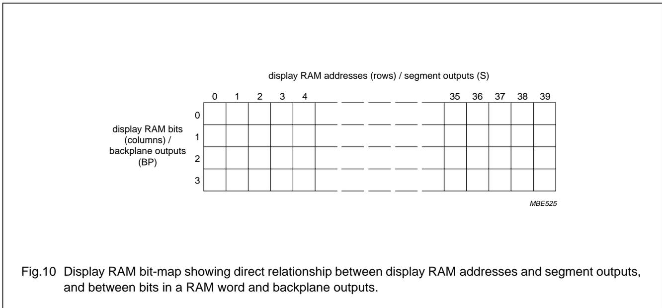
Fig.10 Display RAM bit-map showing direct relationship between display RAM addresses and segment outputs, and between bits in a RAM word and backplane outputs.
