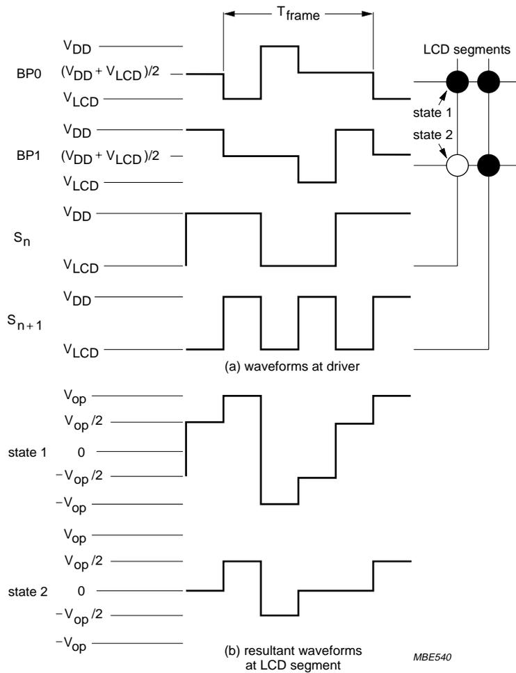
$$V_{state1}(t) = V_{S_n}(t) - V_{BP0}(t)$$
