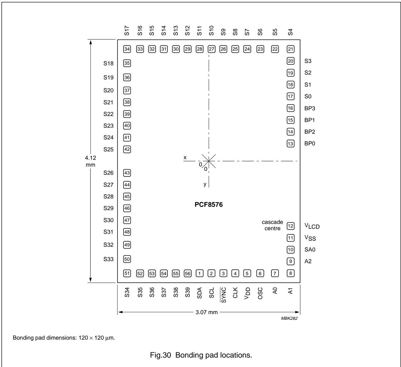
Fig.30 Bonding pad locations.
