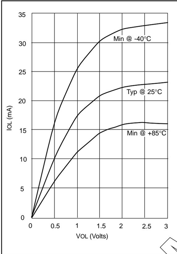
FIGURE 13-21:  $I_{OL}$  vs  $V_{OL}$ ,  $V_{DD} = 5V^*$
