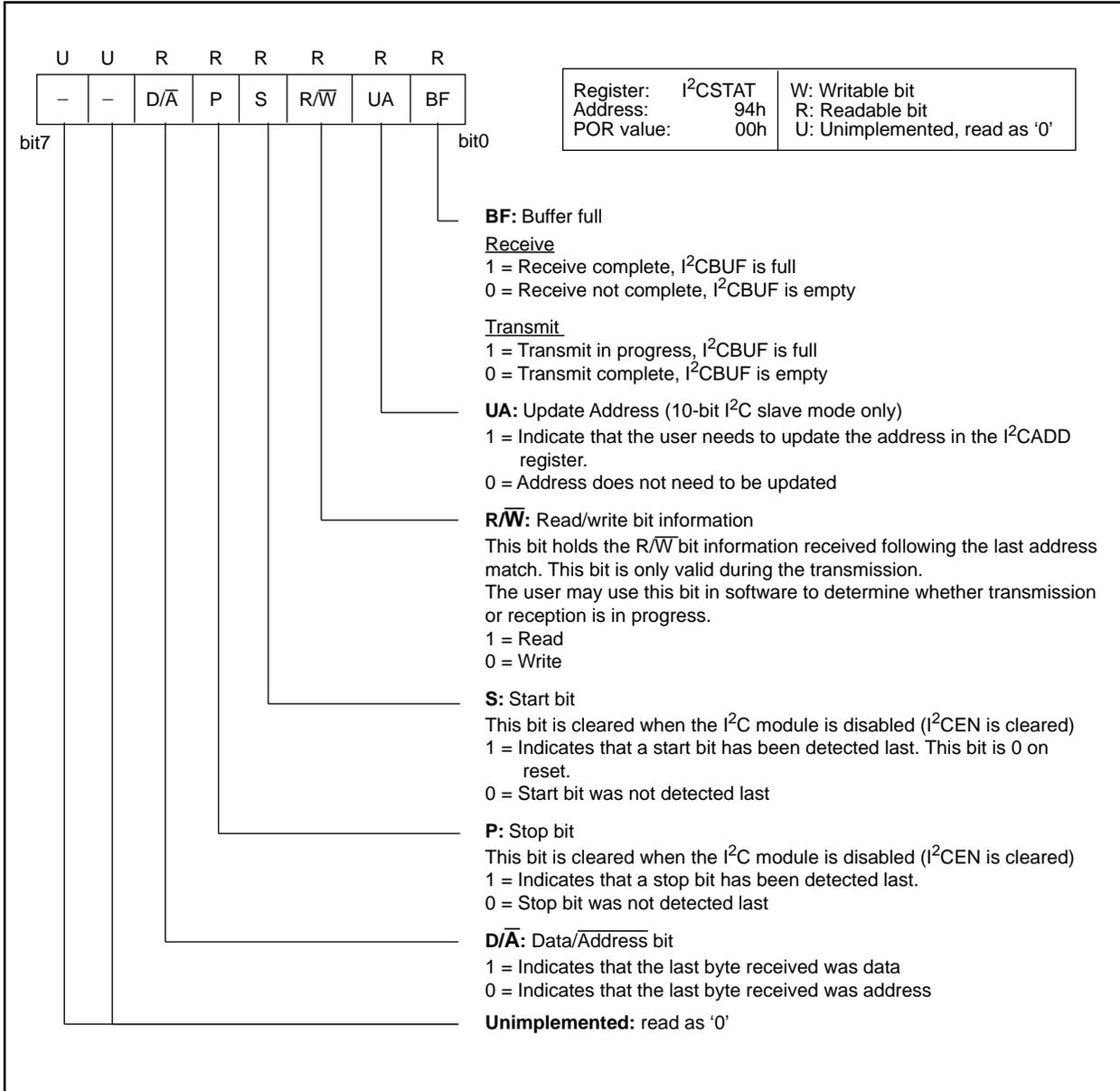
**FIGURE 7-3: I<sup>2</sup>CCON: I<sup>2</sup>C PORT CONTROL REGISTER**
