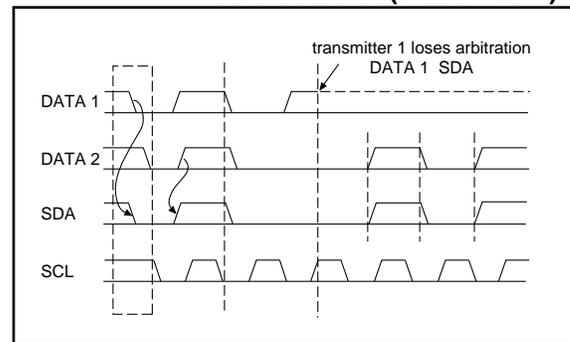
**FIGURE 7-12: I<sup>2</sup>C CLOCK SYNCHRONIZATION**
