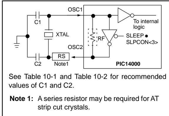
**FIGURE 10-4: EXTERNAL CLOCK INPUT OPERATION (HS OSC CONFIGURATION)**
