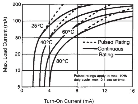
Figure 4. Minimum Control Current for Full Turn-On
