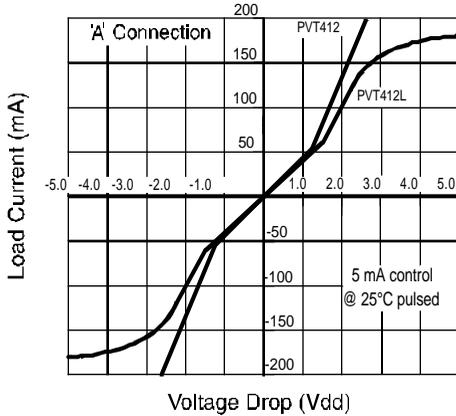
Figure 3. Linearity Characteristics
